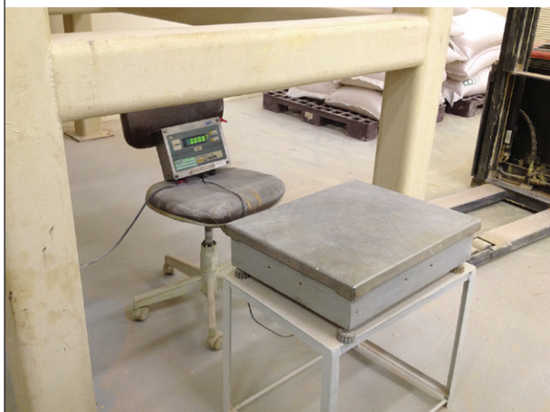
FIGURE 15 Scale not properly placed leading to errors during weighing of ingredients
